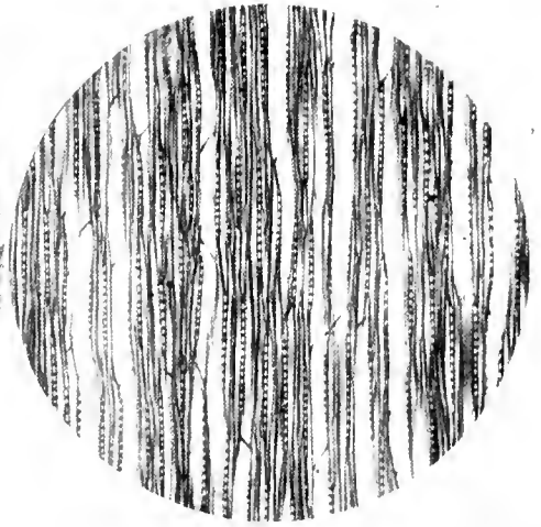
Tangential section of Ohio Buckeye ( Aesculus glabra Willd.), showing typical irregular disposition of rays and vessel segments. Enlarged fifty diameters.
